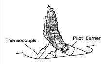
Figure 21 - Incorrect Pilot Flame Pattern
